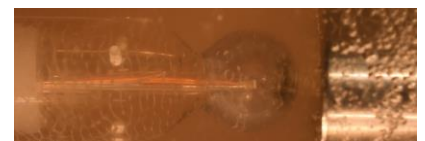
Figure 8: Making the ultrasound field visible with the help of suspended particles: their pattern on the pH-probe reassembles the cleaning force's active area and indicates the range of the cleaning effect
